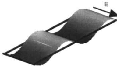
FIGURE.9 Illustration of film vibration
